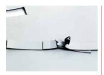
The membrane must fail outside the welding seam.
