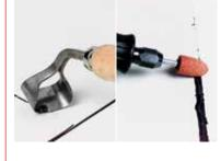
This operation removes the difference in height resulting from the overlapping of several waterproofing sheets and allows adequate cleaning of the seam prior to welding.
