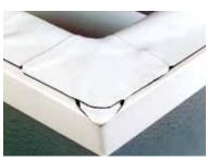
Spot-weld, pre-weld and weld the patch onto the corner.
