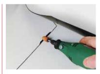
Spot-weld, pre-weld and weld the overlap on the upper edge (B) of the horizontal surface.
